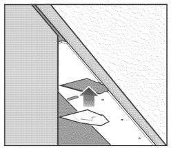
Press the optic indicator reflector in place.
